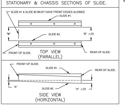
RECOMMENDED TOLERANCE FOR MOUNTING
