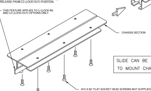
SLIDE CAN BE DISASSEMBLED TO MOUNT CHASSIS SECTION
